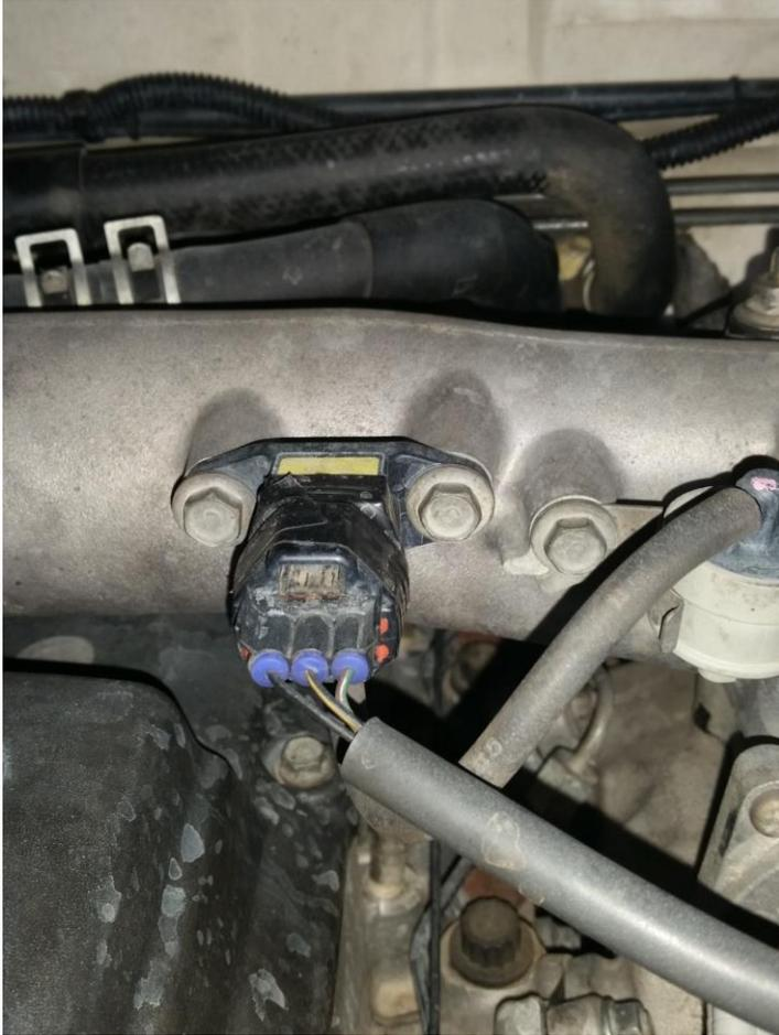
**Photo of Turbo Pressure Sensor.**
