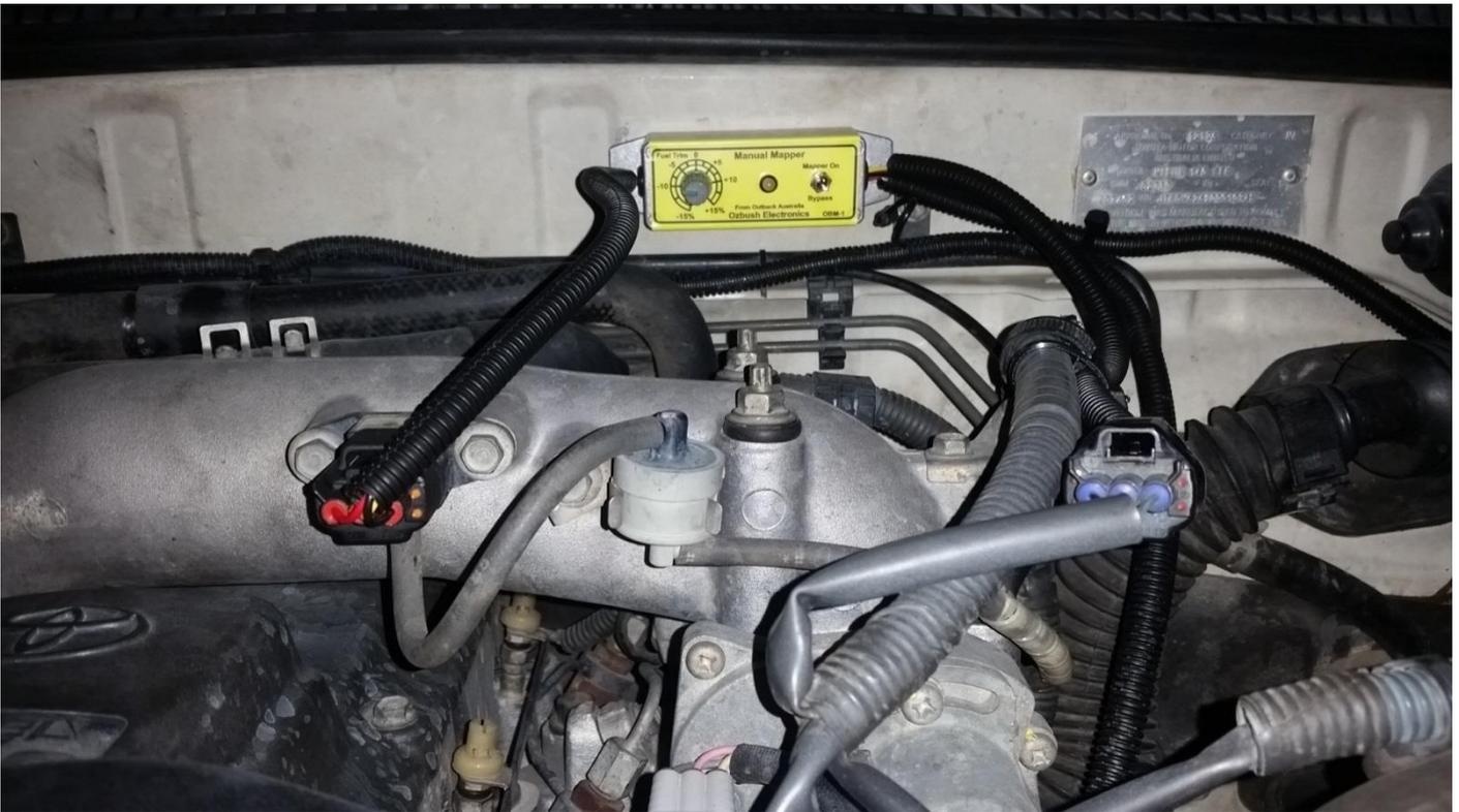
After the installation, check the green light is on when the Mapper is turned on.
