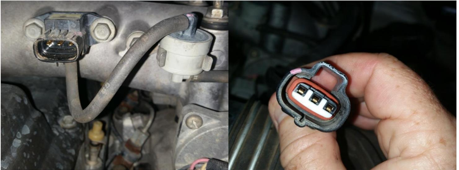
Insert Manual Mapper OBM-2T in between the turbo pressure sensor and car computer.
