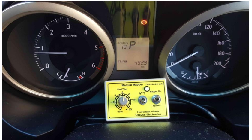
Recommended Position for the Remote Control Box
