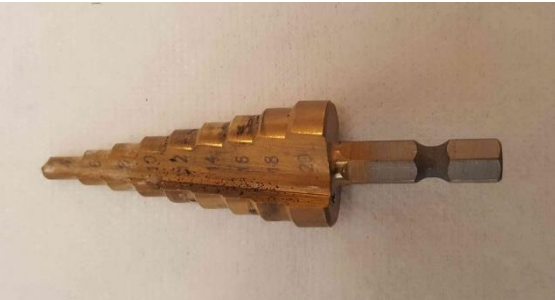
Drill bit for making a large hole
