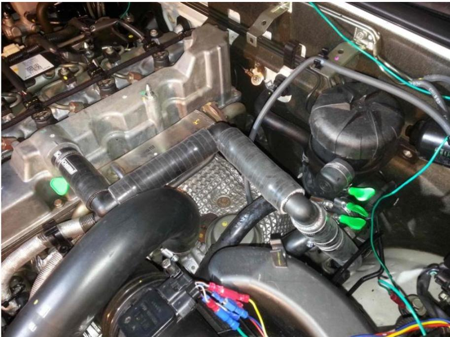
The inlet of the Oil catch can is blocked to stop air leak and against water entering.
