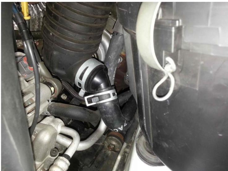
In this photo PCV pipe is connected to oil catch can for deep water crossing.
