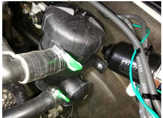
Chair foot is used to block the oil catch can inlet when not used.
